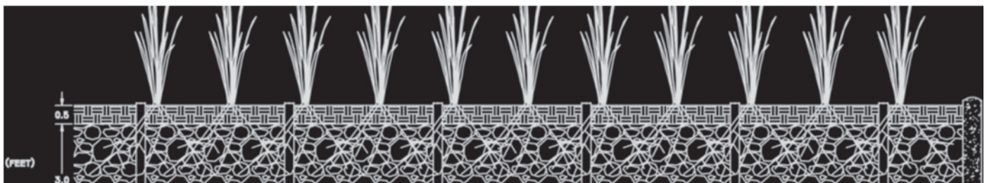
Figure 5: Constructed Wetland Section
